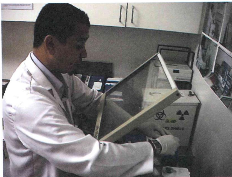
Technetium - 99m Generator Elution/Milking
